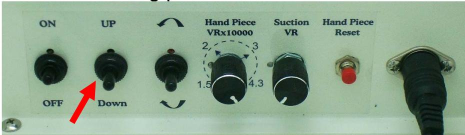
4. Push up or down to select and start the micro motor spin direction CW or CCW.
