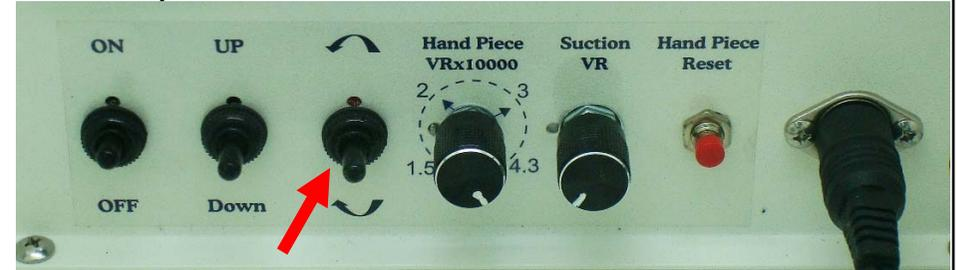
5. Turn the knob to adjust the micro motor spin speed, left for slower and right for faster.
